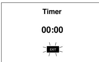
Key in the time required in minutes and seconds, maximum 29 minutes and 59 seconds, using the numerical keys, then press [OK] to start the timer. Use the  $\leftarrow$  and  $\rightarrow$  keys to reposition the cursor and re-enter the time if it is keyed in incorrectly.
