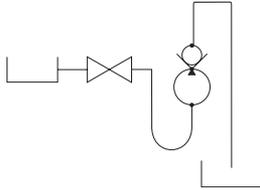
It is important to install the Injection valve to prevent siphoning.
