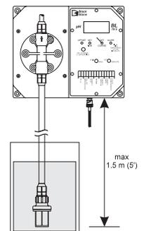
For the U.S. standard installations, use PVC adapters to connect the suction and discharge valves to the PVC pipe.
