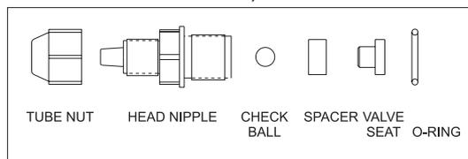
**HI721103** Suction Valve (Glass Ball, Valve O-Ring, Hose Connector)
