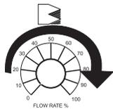
4. Switch the pump ON to the estimated setting and run for a specific amount of time (e.g. 1 minute). Count the number of strokes, length of time, and volume pumped.
