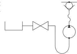
A slight suction pressure avoids self-priming problems, especially with high viscosity liquids.
