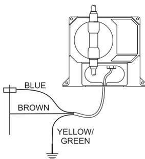
It is recommended that the system be connected to a power line/leg equipped with a circuit breaker of 1 Amp.
