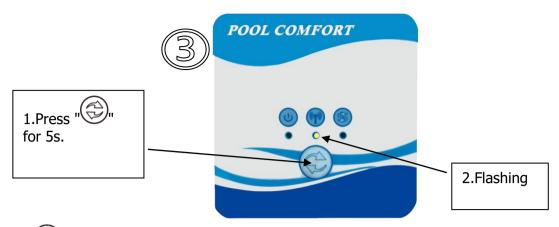
Press "for 5s to enter the distribution network. When entering, the "icon light flashes quickly.( If this light is flashing, skip this step.)
