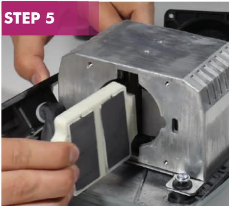
Remove one of the magnet bar ends by pulling it out of the housing, being careful not to scratch or break the housing or magnet bar.
