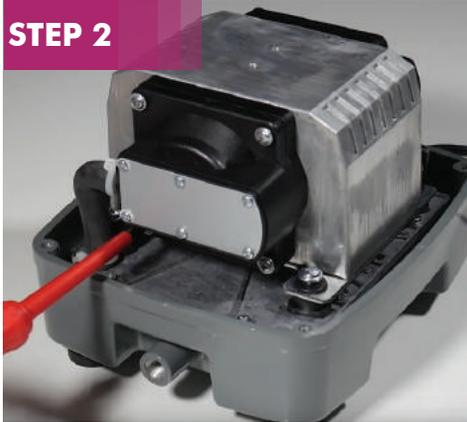
Unscrew the four corner screws from the chamber cover at one end of the pump. Separate the chamber cover at the seam to expose the screw holding the white round plastic diaphragm depressor in place.
