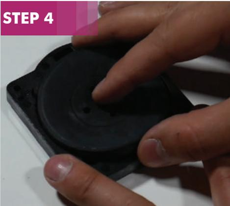
Replaced both diaphragms with new ones provided in your service kit, ensuring the edges are fully pushed into the grooves of the frame.
