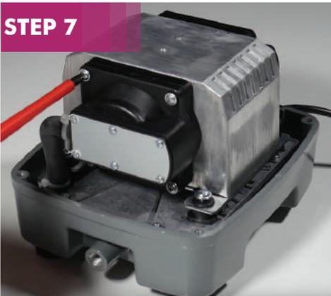
Put chamber cover back and screw four screws in. Repeat this process on the opposite side of the pump.
