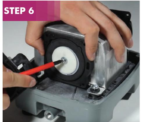
Gently slide in the new magnet bar from the kit. Put on the end cap, the first electrostatic membrane, diaphragm, second electrostatic membrane, diaphragm depressor and use single screw to hold in place.
