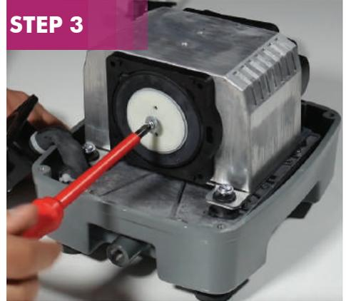
Remove the screw along with the diaphragm depressor, electrostatic membrane and diaphragm. Repeat on the opposite end of the pump.
