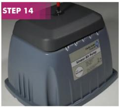
To change the filter unscrew the pump lid.
