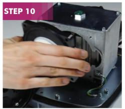
Remove the diaphragm frame and peel off the worn diaphragm.
