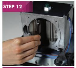
Remove the worn magnet and replace with the new one provided.
