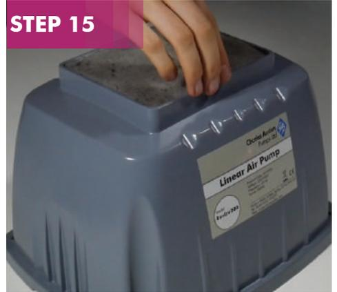
Remove the dirty filter and clean away any dust or dirt that has been collected.
