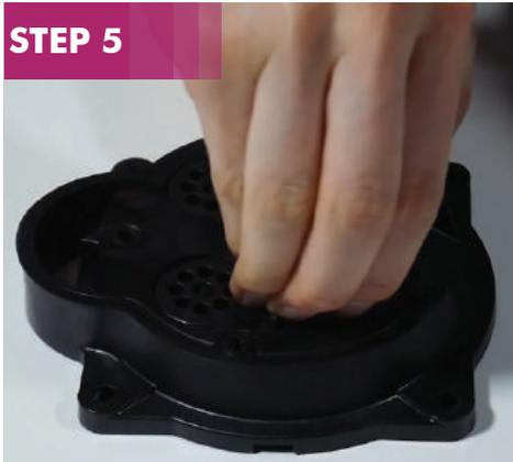
Remove the valves from the chamber block, take note of the valve formation.
