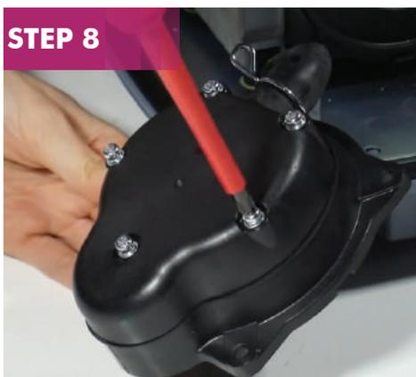
Screw the chamber block back together ensuring the rubber seal between them lined up properly. Repeat this process on the opposite side of the pump.
