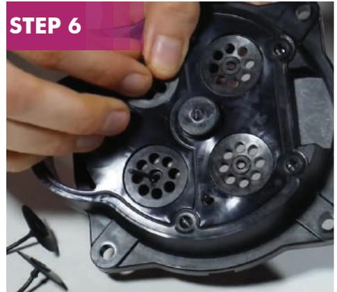
Pull the new valves through, you should hear a 'snap' sound once secured in place.
