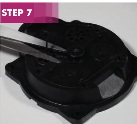
Cut the excess rubber off from the valves and discard.
