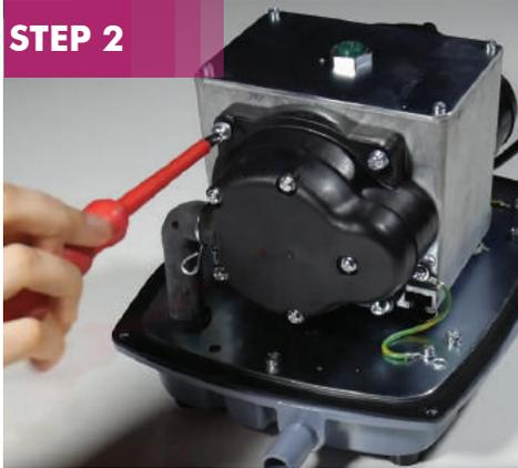
Unscrew the chamber cover at one end of the pump. Separate the chamber cover at the seam to expose the screw holding the white round plastic diaphragm depressor in place.
