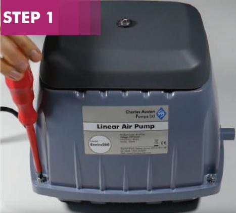
To start, unplug the pump from the mains. Unscrew and remove the cover from the air pump.
