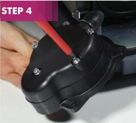
Unscrew the chamber block and pull it apart.
