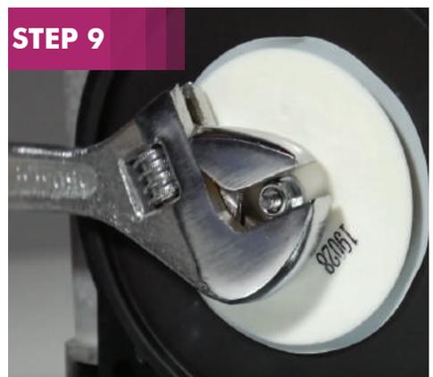
Undo the bolt from the diaphragm.
