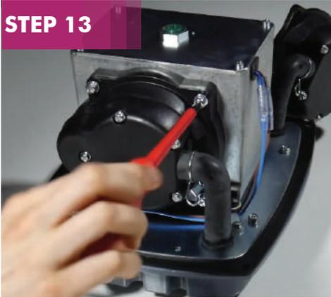
Connect the chamber block and diaphragm together and screw back into place. Repeat on the opposite side of the pump.
